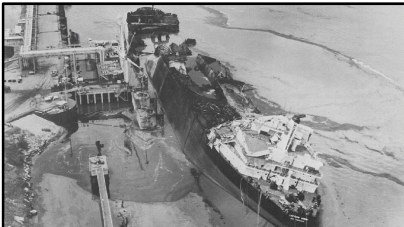
The Chevron Hawaii following the explosion at the Deer Park Terminal on September 1, 1979. There were three fatalities and the explosion caused by a lightning strike resulted in secondary explosions in a land-based storage tank and three adjacent barges.
